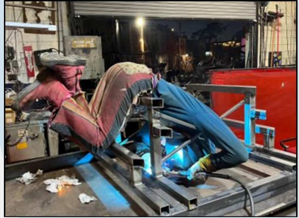
Awkward welding positions
