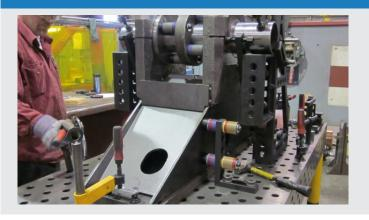
Welding their truck axle mounts on a Bluco modular fixture allowed this manufacturer to deliver better quality parts in less time. The modular table base and CAD templates make it easy to set up and change over fixtures quickly and accurately. The adjustable axle simulator not only maintained hole alignment, it also served as a constant QC device, and made it easy to tip and unload the part for weld out, making final assembly that much easier.
