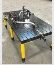
A single modular fixturing solution can be used for virtually any exhaust platform, eliminating the repeated expense and expanding space needed to build and store the dozens of dedicated fixtures that used to be needed. The templates and digital instructions provided by Bluco engineers help cut fixture design and build time significantly. Plus, modular versatility makes finetuning easy, resulting in a more accurate and faster prototyping process for this manufacturer.
