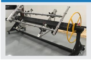
The build starts by loading pre-tacked burner tube assemblies into the fixture and securing with clamps. No CAD models or set-ups are needed. The operator simply moves the outriggers to wherever they're needed to support the assembled tube. The Manual Positioner allows ergonomic lift and manual rotation for limitless positions and easy assembly of deflectors. No more saw horses. No more crouching, bending or rolling sharp-edged parts by hand.
