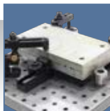
Highlighted parts from the same 142-Piece kit are used to build this fixture.
