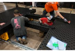
The new Bluco solution was assembled with the help of Bluco engineers using CAD models. It included 5 tables and 12 meters of floor rail.
