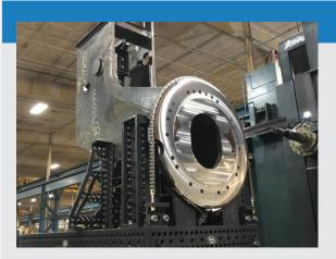
Fixturing the part properly for machining provided the rigidity needed speed up the machine. In addition, the part could be setup offline and set on the mill. This reduced machine downtime and also eliminated the need to assemble the fixture on the machine bed — a slippery place to work. The results were faster fixturing, more accurate results, higher throughput and a very happy machine operator.
