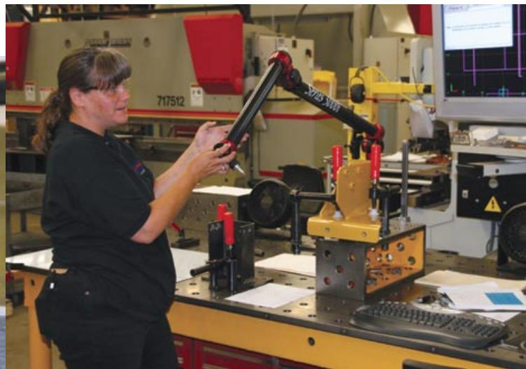
Articulated arm ergonomics offers enhanced productivity. The operator is using the arm-end as a mouse to position the cursor directly on the display screen to select datums for measurement. Triggering the probe generates the click. Used as a mouse, the arm-end can control many functions of the arm's metrology program. Source: *Bluco*
