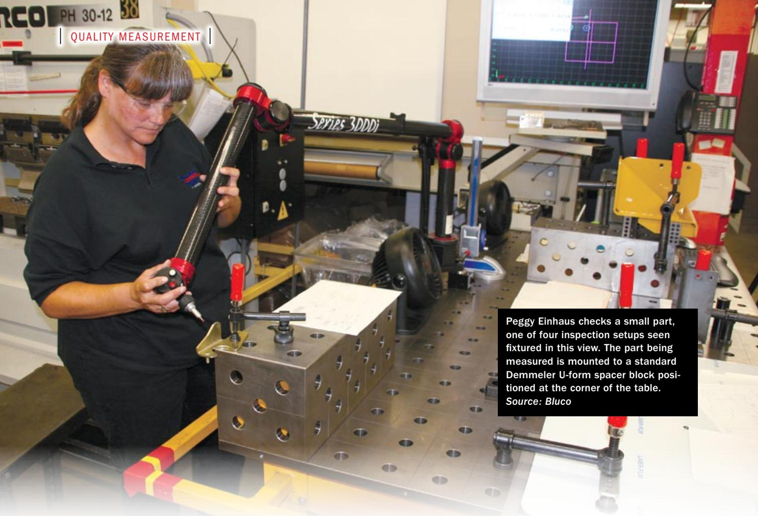
Peggy Einhaus checks a small part, one of four inspection setups seen fixtured in this view. The part being measured is mounted to a standard Demmeler U-form spacer block positioned at the corner of the table.
