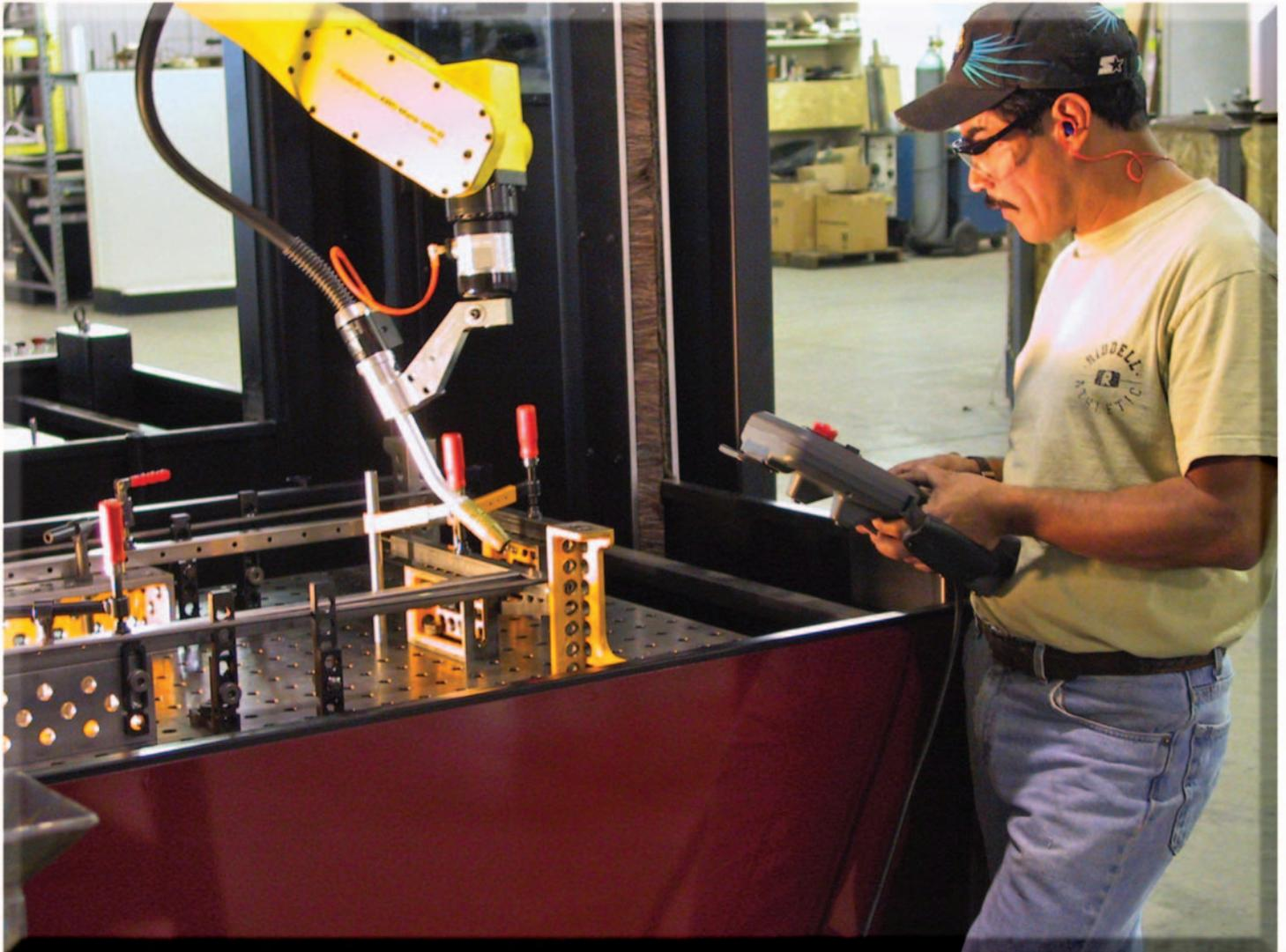
*A Keystone employee brings the robot into position to check clearances in preparation of the weld sequence.*
