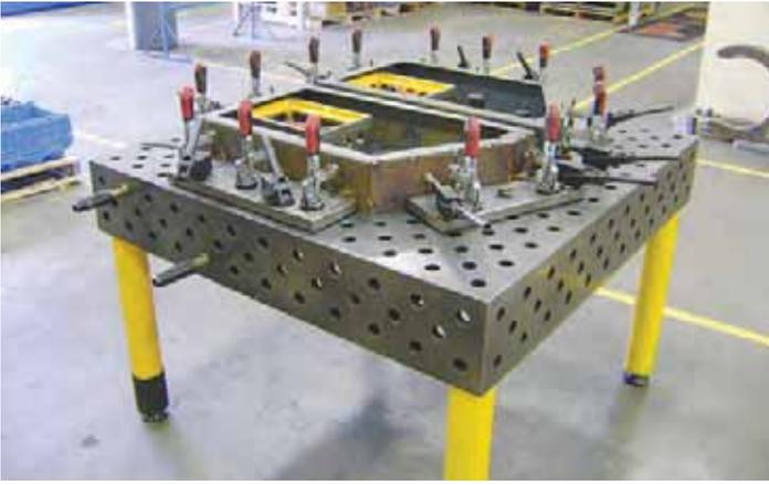
**Modular fixture built from the CAD model.**
