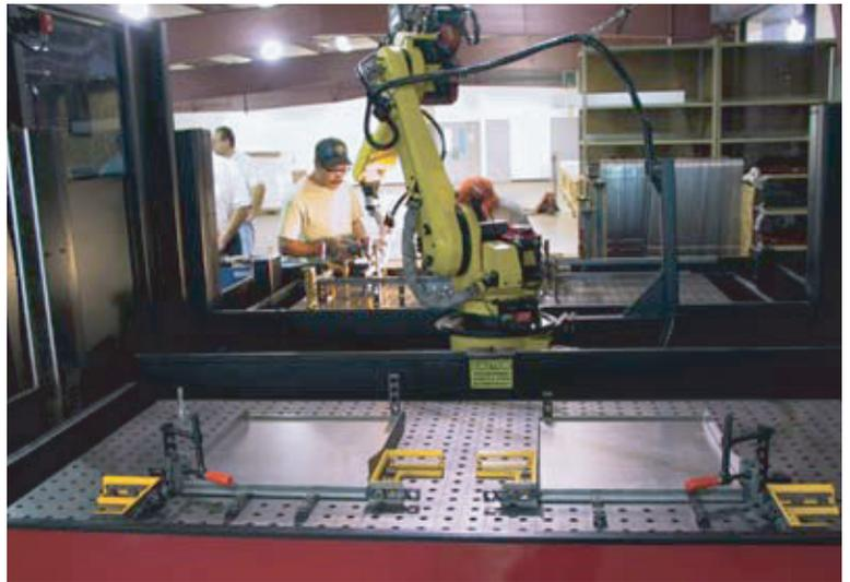
A setup operator builds a modular fixture and teaches a robot the program.
