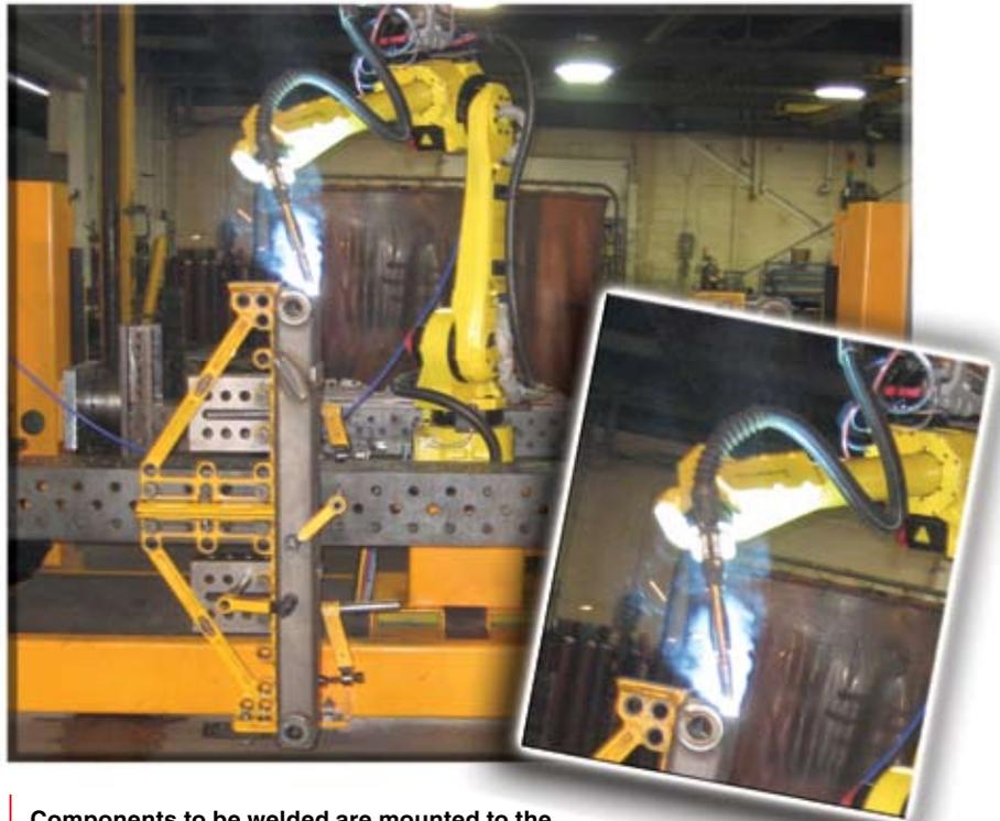
**Components to be welded are mounted to the Bluco beam using angles, blocks, and other elements. The two beams then rotate, providing the robot welder with access to the surfaces, allowing all of the welds for two assemblies in one operation.**
