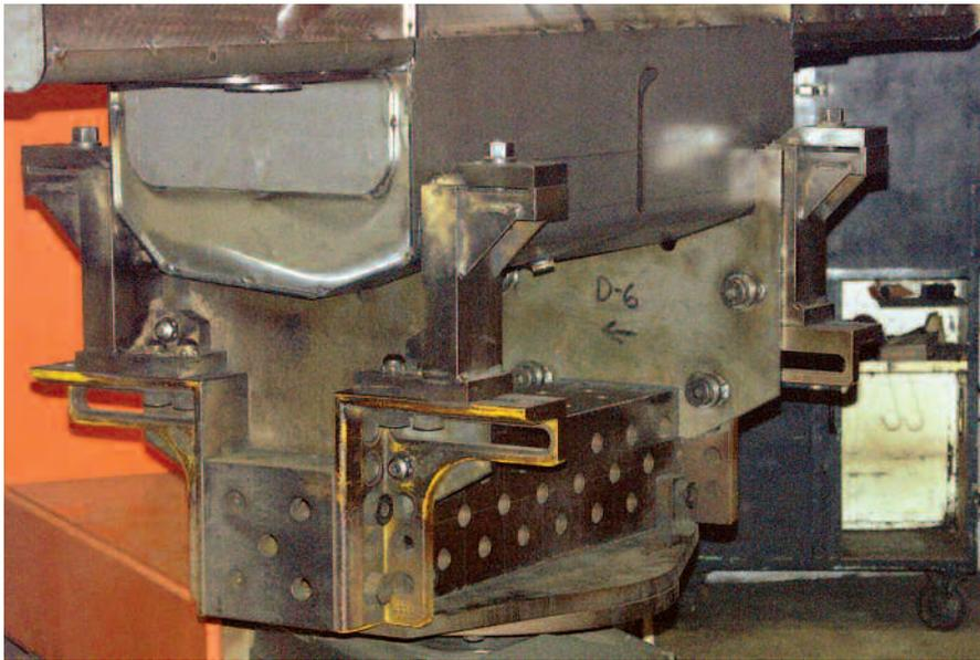
▲ **FIGURE 1** Fixturing needs to be rigid and accurate to handle positioner rotation.
