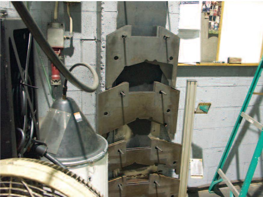
▲ **FIGURE 2** Special laser-cut fixtures are prepared for each different part.
