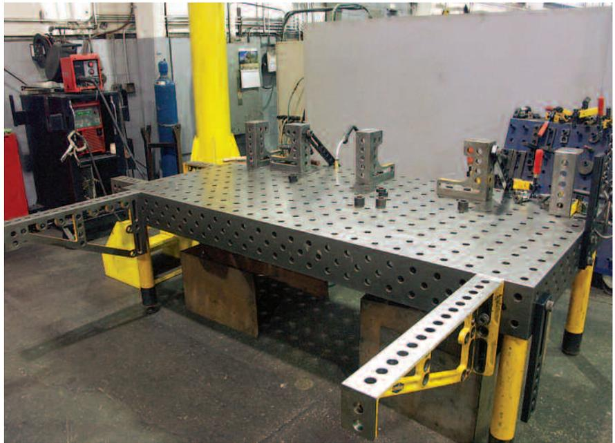
▲ **FIGURE 3** The table is five-sided with a pattern of bores on all four sides to accommodate parts larger than its surface. For example, a 4-ft.-wide table with an extension can accommodate 9-ft.-wide parts.
