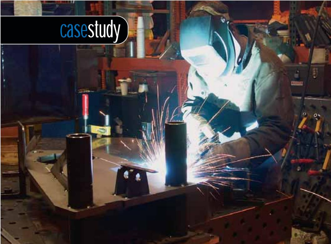
Sitting on top of a modular fixturing table, a rock wheel frame attachment for a skid steer is finish-welded.
