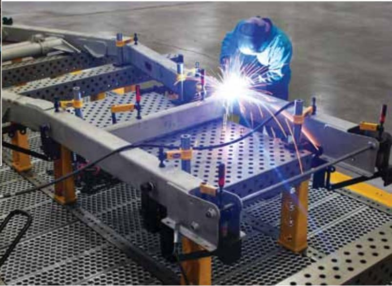
Figure 4. In a modular system, the rails with the same pattern of bores as the tables are lagged to the floor, precisely spaced and leveled for handling large parts. A combination of tables with special spacer frames and narrower bridges with the same pattern of bores as the tables can be used to hold and locate large parts.
