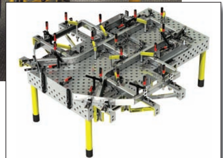
Bluco Corp. will design a fixture for a typical part to show customers what table accessories are needed for a specific job.
