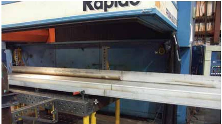
**Northern replaced the laser's table with a 5 × 10' Demmeler table to handle the longer part, which is indexed after one section is welded to complete the welding operation.**
