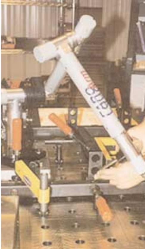
Ron Woodard verifies both the fixture and the welded workpiece with a table-mounted CMM.
