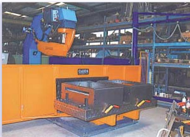
**Robot with a pallet changer allows robot to run while the welder sets up the next part.**
