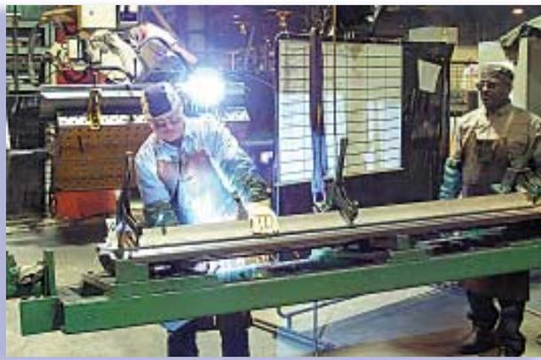
**Loose workpieces are assembled outside the robot welding area, using a customer-supplied dedicated fixture to tack-weld parts in an initial stage.**
