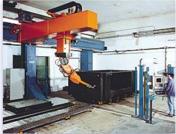
**For larger parts, a gantry robot has two Demmeler tables as floor plates.**
