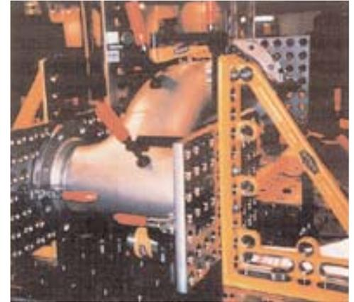
Manifold and pipe flanges for welding
