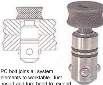
PC bolt joins all system elements to worktable. Just insert and turn head to extend balls in shank and provide 5-ton clamping force, 25-ton shear force. O-ring keeps bolt from turning during tightening, permitting one-hand operation.
