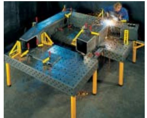
Connected worktables support machine-gantry frame section during welding
